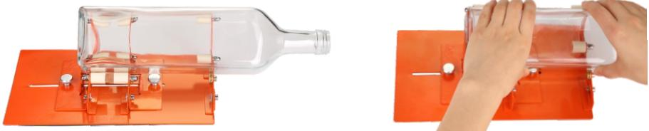
(3)Now etching the flat surfaces of bottle. When you etch the flat surface of the square bottle, Place the blade vertically so that the blade always remains in contact with the glass.
