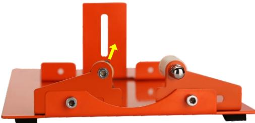
(2)Just etching the corners of bottle firstly, apply constant pressure as you rotate the bottle towards one direction with two hands. Rotate it slowly as the blade rolls over the corners of the square bottle. Keep it firmly against the backstop and keep it moving while you're making the etching.
