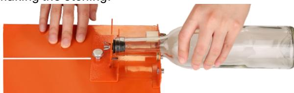
**Tips:** Before removing the bottle, please make sure that the distance between the cutter and roller is wide enough.
