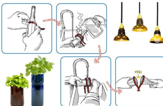
(1) Rinse the etching mark with almost boiling water and rotate the bottle at a faster pace to give a uniform temperature to the glass. (Look out that hot water might hurt you). The bottle should feel hot to the touch, but not too hot to handle.
