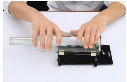
(2) Rotate the bottle toward one direction with two hands. Keep it firmly against the backstop and keep it moving while you're making the etching.
