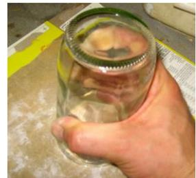
(3) Dip the edge of the glass in water and then place it on the polishing surface. Start to grind in a circular motion. After a short time, the edge of the glass will become perfectly flat and have a dull, gray appearance.
