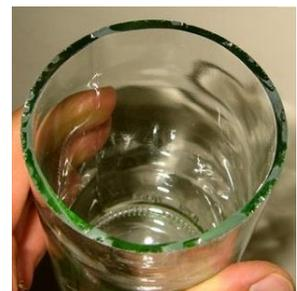
(4) Again, smooth the inside and outside edges with the polishing paper. The finer polishing paper should be used to give a final smooth finish. Use water on the paper periodically while polishing.
